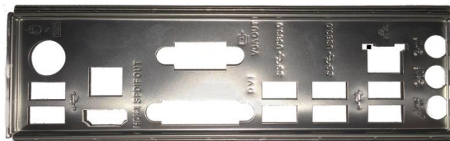
Figure 1 Example I/O panel
